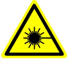
**CLASS 2 & 4 LASER IN USE.** Exposure to laser beam may cause physical burns and severe eye damage. Do not stare into beam directly, or with optical instruments. Serious and permanent damage may result to optic nerve, cornea or lens due to improper use. Immediately stop use and seek medical attention if you begin seeing spots or experiencing blurred vision.
