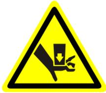
**MOVING COMPONENTS POSE CRUSHING HAZARD.** Do not reach into the build area during printing or warm-up. Keep hands clear of moving components at all times. Disconnect power before proceeding with maintenance. Failure to comply may result in serious injury.
