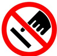
**DO NOT TOUCH OPTICAL WINDOWS ON PRINTER OR RESIN TANKS.** Avoid touching the windows on the printer and the resin tanks at all times, even with gloves. Hold resin tanks by the brims along the left and right sides, never from the bottom. Always set tanks down on a level clean surface.
